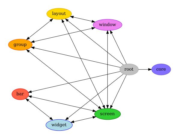
Each arrow can be read as "holds a reference to". So, we can see that a widget object *holds a reference to* objects of type bar, screen and group. Lets start with some simple examples of how the addressing works. Which particular objects we hold reference to depends on the context - for instance, widgets hold a reference to the screen that they appear on, and the bar they are attached to.
