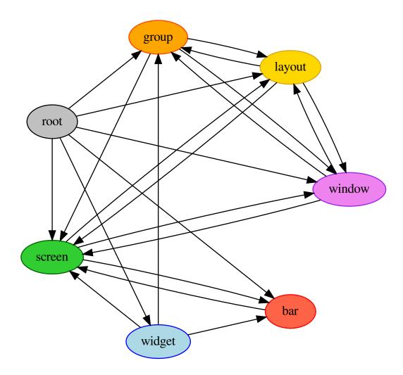
Each arrow can be read as "holds a reference to". So, we can see that a widget object holds a reference to objects of type bar, screen and group. Lets start with some simple examples of how the addressing works. Which particular
