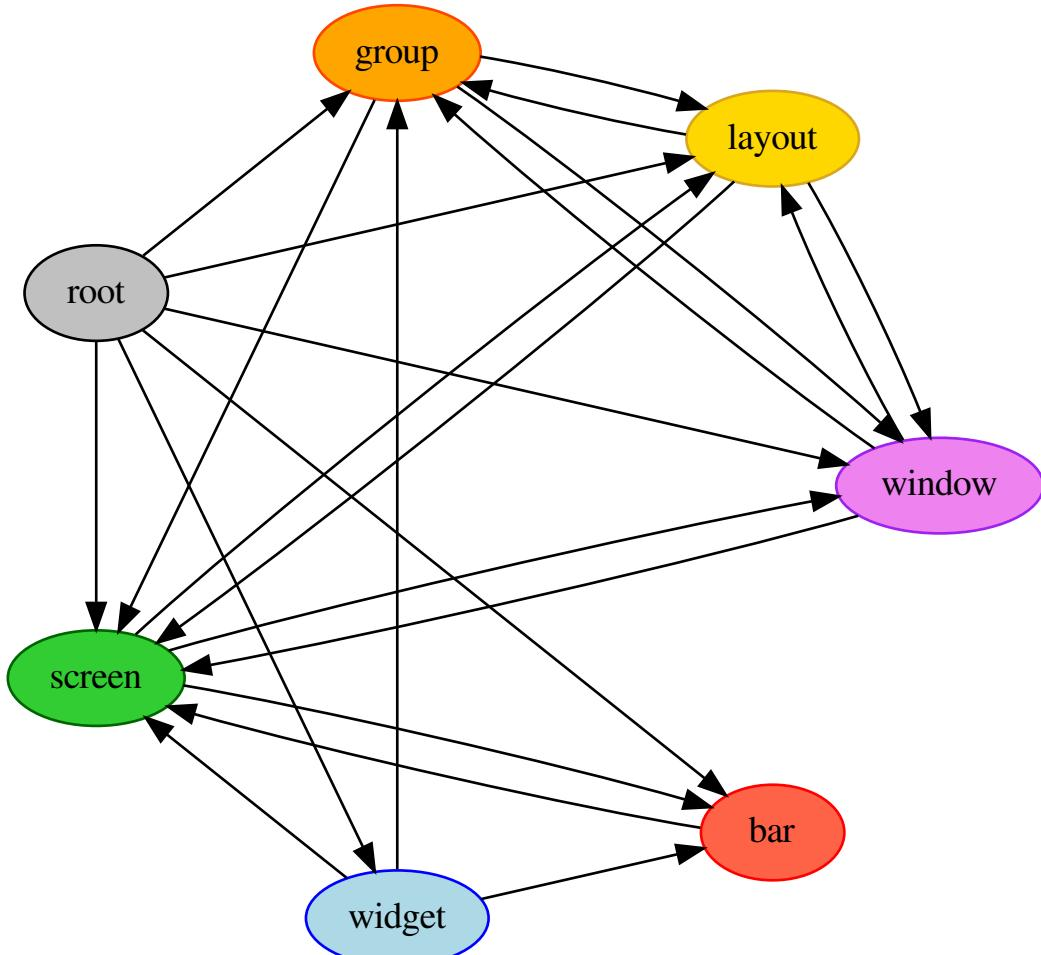
Each arrow can be read as “holds a reference to”. So, we can see that a `widget` object *holds a reference to* objects of type `bar`, `screen` and `group`. Lets start with some simple examples of how the addressing works. Which particular objects we hold reference to depends on the context - for instance, widgets hold a reference to the screen that they appear on, and the bar they are attached to.
